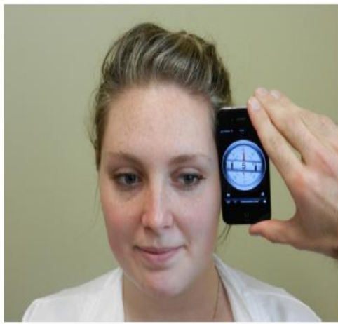
Figure 2 Position of the iPhone for the measurement of right lateral flexion. (1) Starting position. (2) Position at end range of right lateral flexion. The iPhone's level is aligned with the corner of the eye.
